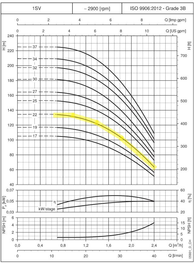
These performances are valid for liquids with density  $\rho=1.0$  Kg/dm³ and kinematic viscosity  $\nu=1$  mm²/sec.
